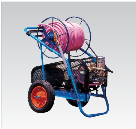
High pressure washer(movable) - work. pr/max.pressure(kg/cm 2 ) : 15/55 - Water(ℓ/min) : 20/50 - Motor : 2.2kw (Single phase) 3.7kw (3 phase) - Power supply : Single phase, 220V 3 phase, 220/380V - Weight: 90kg - Size(L×W×H) : 950×640×930mm
