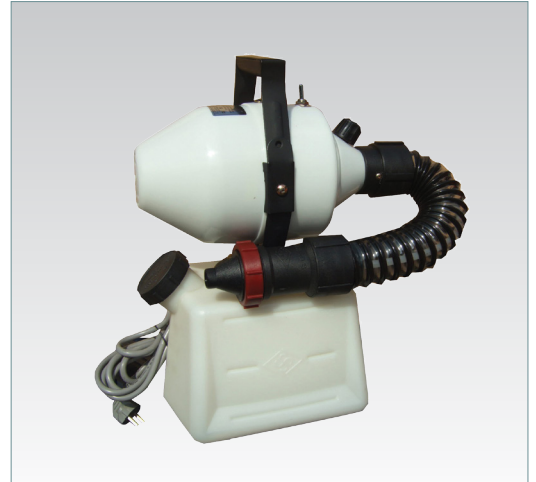
SS-20EU - AC220V, 20000RPM - Injection rate=20ℓ / h, Chemical tank=6ℓ - Size(L×W×H) 320×200×420mm (Weight=4.5kg)
