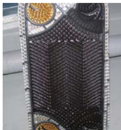
Not inputting the pipe cleaning agent
