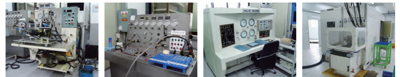
Valve Test Stnad 210kg/cm 2 , 20Lpm Valve Test Stnad 350kg/cm 2 , 80Lpm Proportional / Valve Test Stnad Pump Test Stnad
